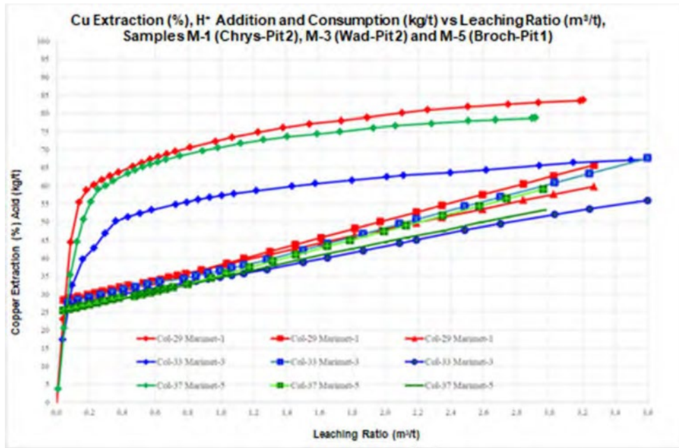
Figure 13-2: Cu Extraction (%), Starting H + Addition in Agglomeration and Consumption (kg/t) vs Leaching Ratio (m 3 /t), M-1, M-3 and M-5.
