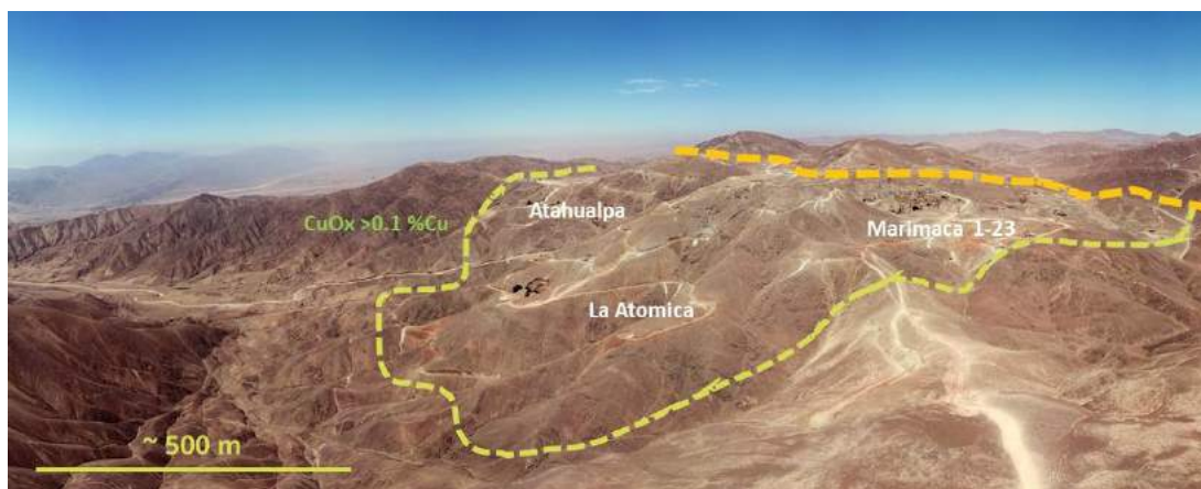
Figure 6-5 Marimaca Project Area. Panoramic view toward north-east showing main sectors and Key elements of copper oxide mineralization (the >0.1% Cu boundary) and alteration (Hanging Wall Front). Scale bar is for reference only. The highest peaks are 1,100 m elevation, lowest are close to 900 m elevation.
