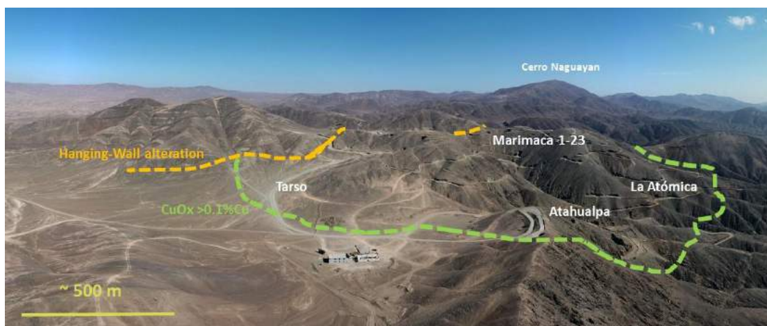
Figure 6-6 Marimaca Project Area. Panoramic view toward south showing main sectors and key elements of copper oxide mineralization (the >0.1% Cu boundary) and alteration (Hanging Wall Front). The northern limit of mineralization corresponds to a NW fault that can be easily observed at the hill above Hanging Wall Alteration. Scale bar is for reference only. Altitude references are same as Figure 6.5.
